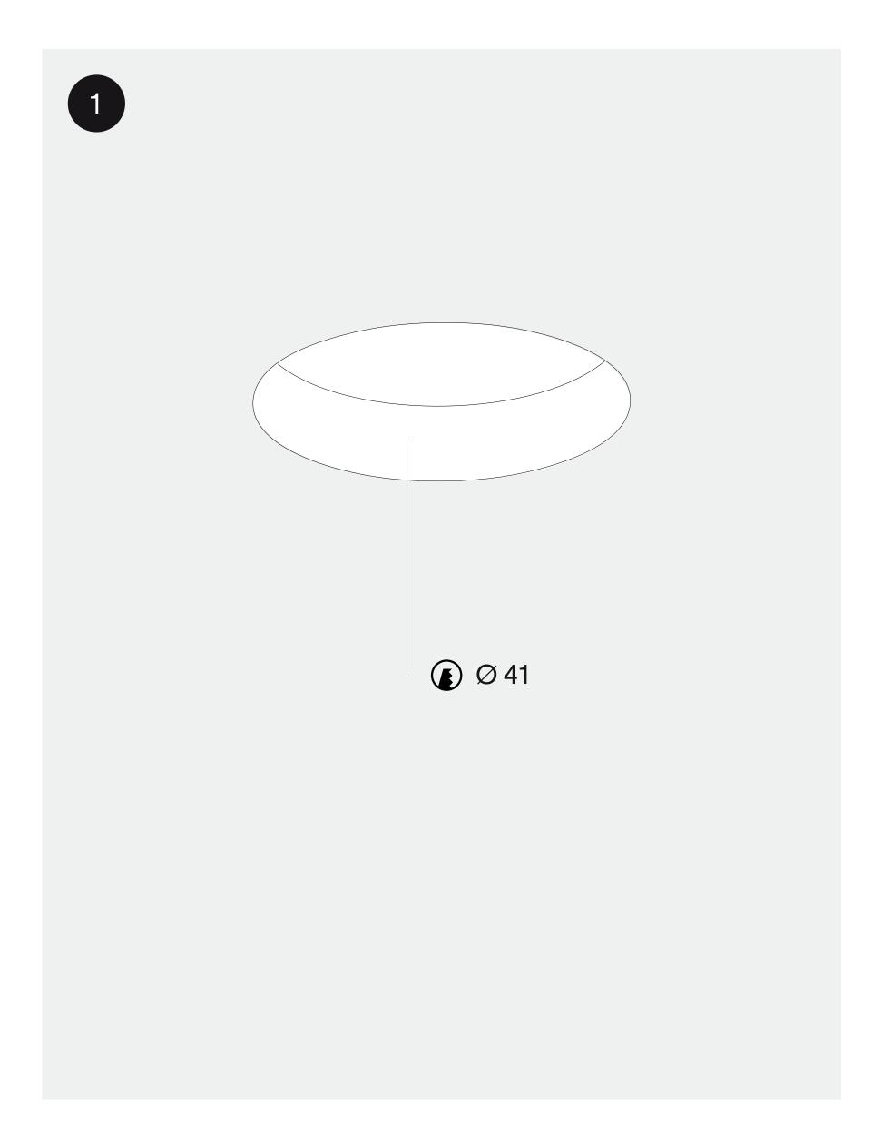
Cut a round hole ( $\emptyset$  41). Consult the chosen luminaire tech specs for required height and free air dimensions.
