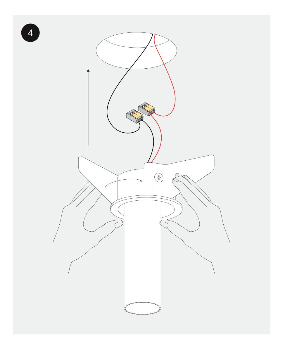
bend over the springs and push the luminaire into the
