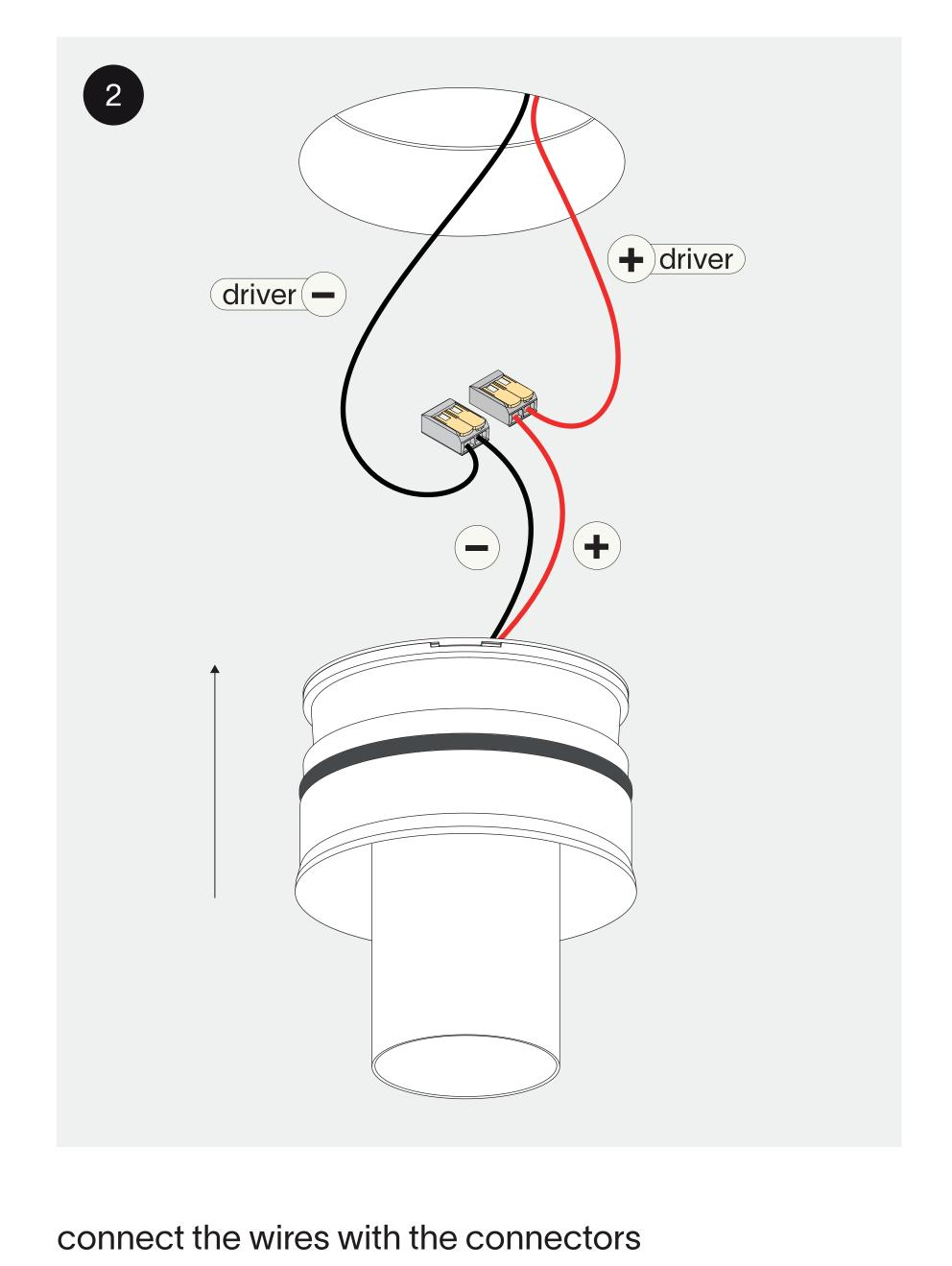
for serial connection, respect polarity
