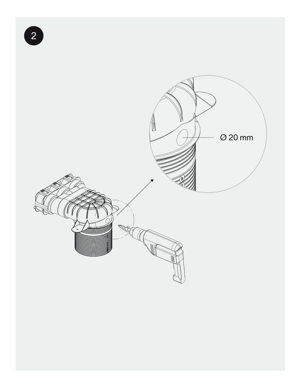
Use a step drill to cut a Ø20 hole into the Ø125 valve adapter of your choice. A hole can be drilled in any type or brand of Ø125 valve adapter.
