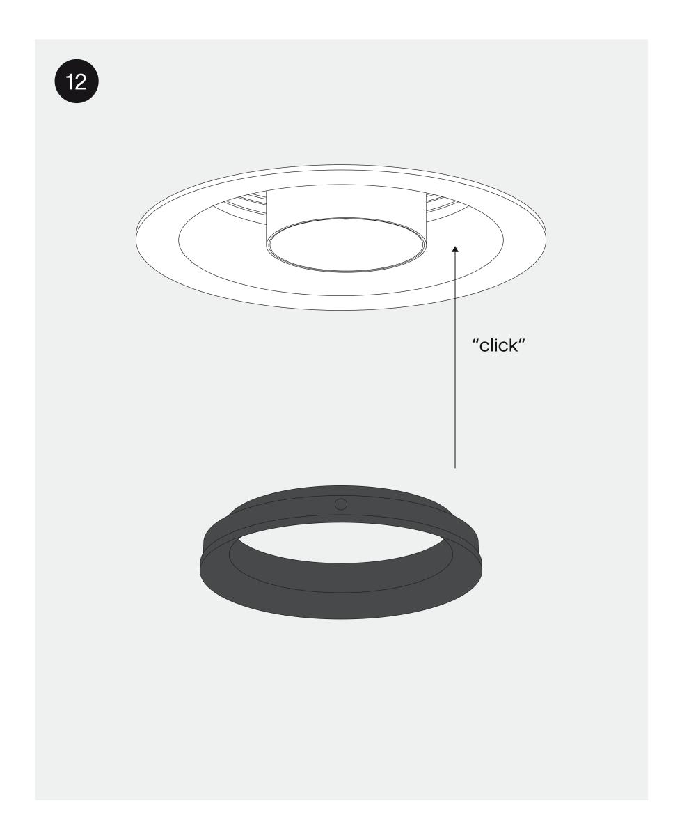
insert the design ring to lock the ventilation valve
