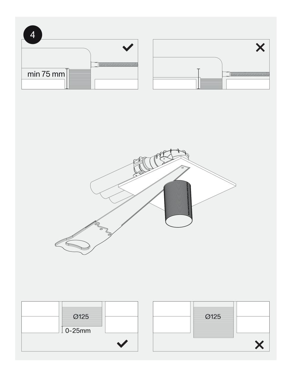
Cut off the excess length of the valve adapter. (between 0 and 25 mm above final ceiling level)
