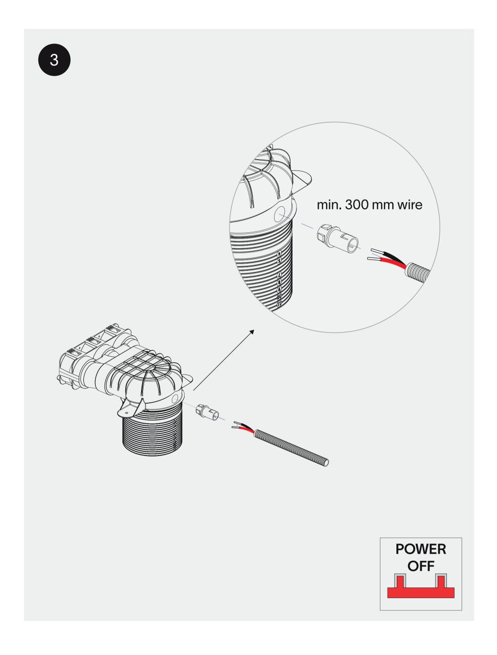
Connect the Ø16 preflex and the valve adapter with the prado connector. Make sure to add minimal 300 mm of wire into the valve adapter.
