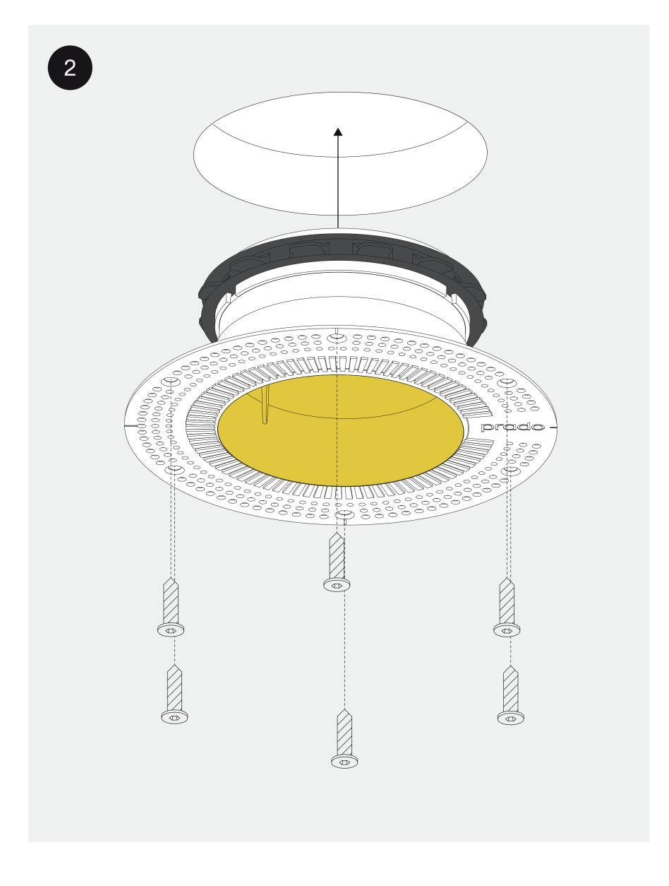
Insert the plaster ring and securely fasten it with glue or the appropriate screws on a screwfast surface. The attachment must be able to obtain a static load of 5 kg. It's the installers responsability to ensure optimal attachment.
