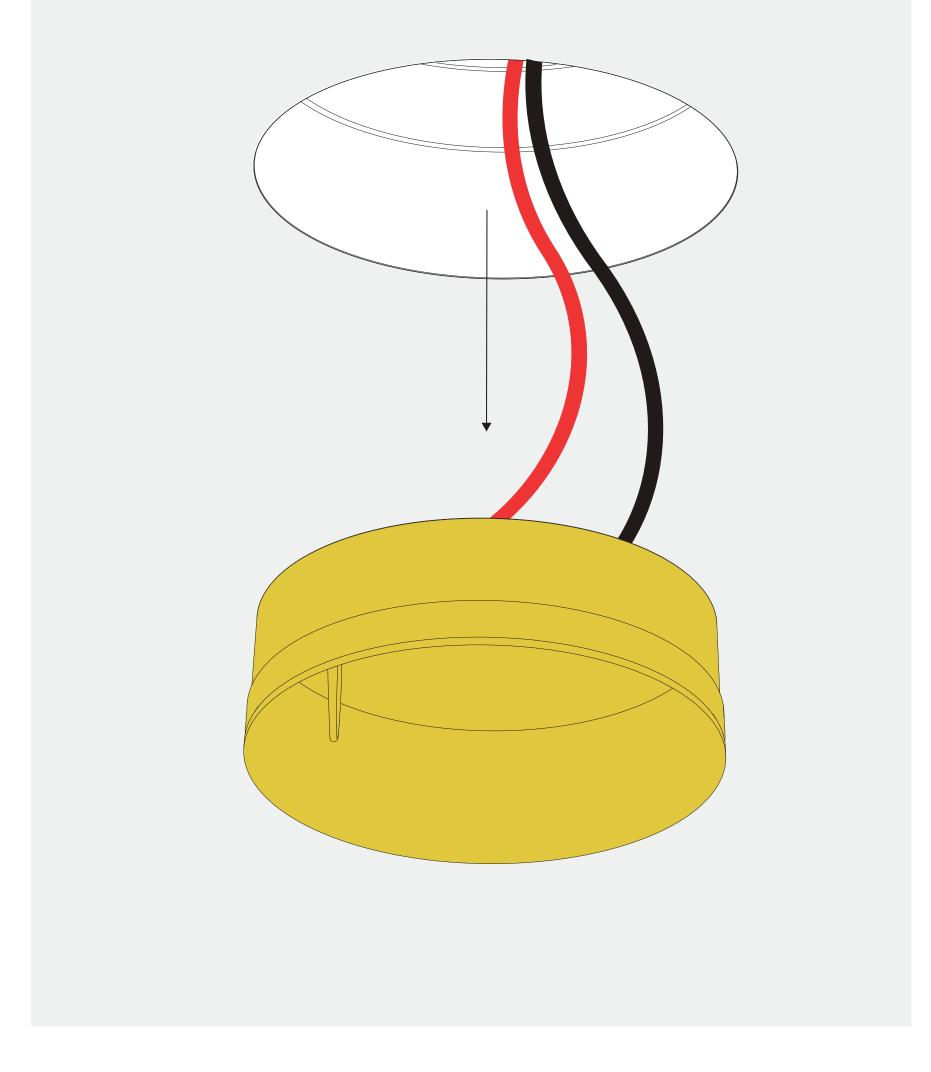
Remove the plaster lid just before installing the fixture. It helps to keep the inside of your plaster ring free of filler, paint and dust. Any residue needs to be removed without damaging the edges of the plaster ring. thank you for choosing prado
