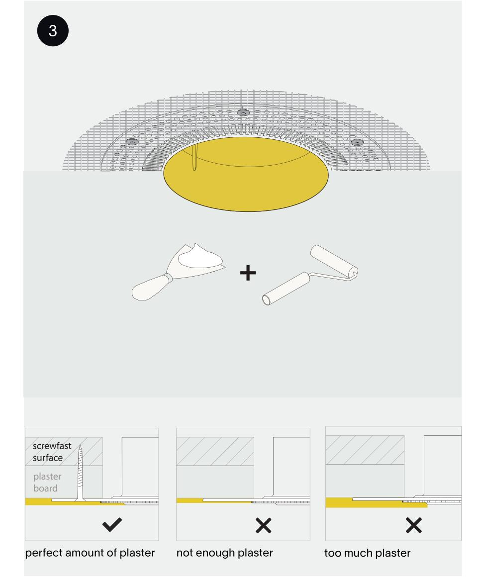
Excercise caution while plasering, do not damage the ring. Keep the plaster lid inside the plaster ring while plastering. Use a fiberglass mesh tape for optimal plaster adhesion. Make sure not to touch the edge of the ring when sanding.
