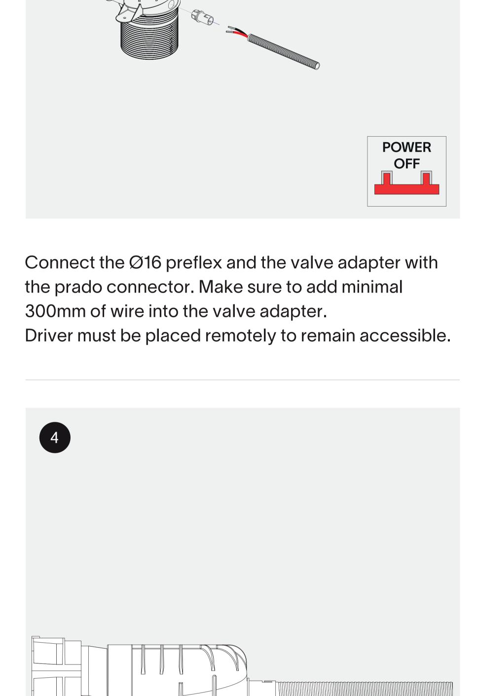
Cut off the excess length of the valve adapter.
