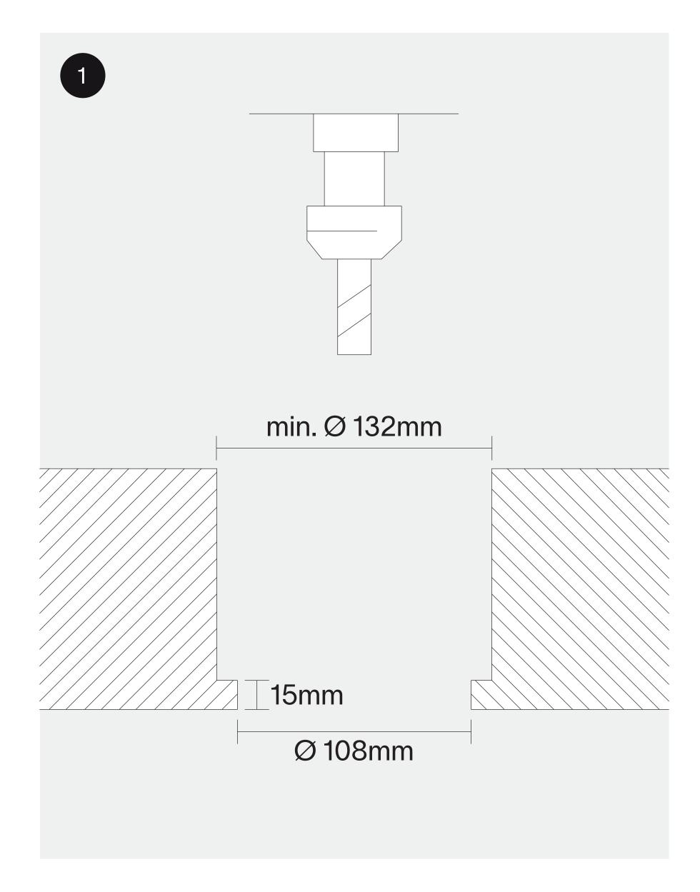
Mill a hole in the CLT ceiling with the above dimensions.
