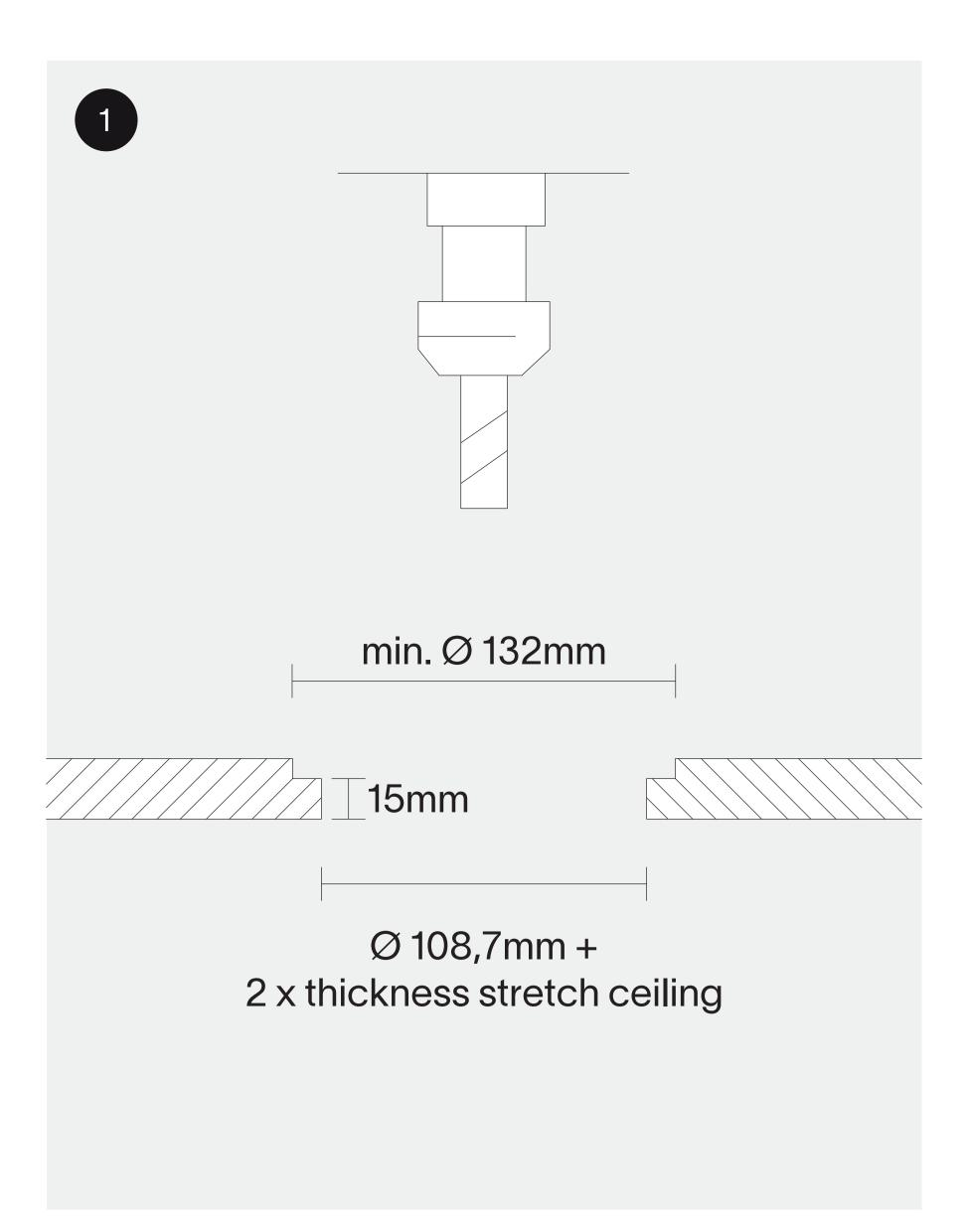
mill a hole with the above dimensions in a wooden base (not supplied) (maximal fabric thickness : 0.6mm)
